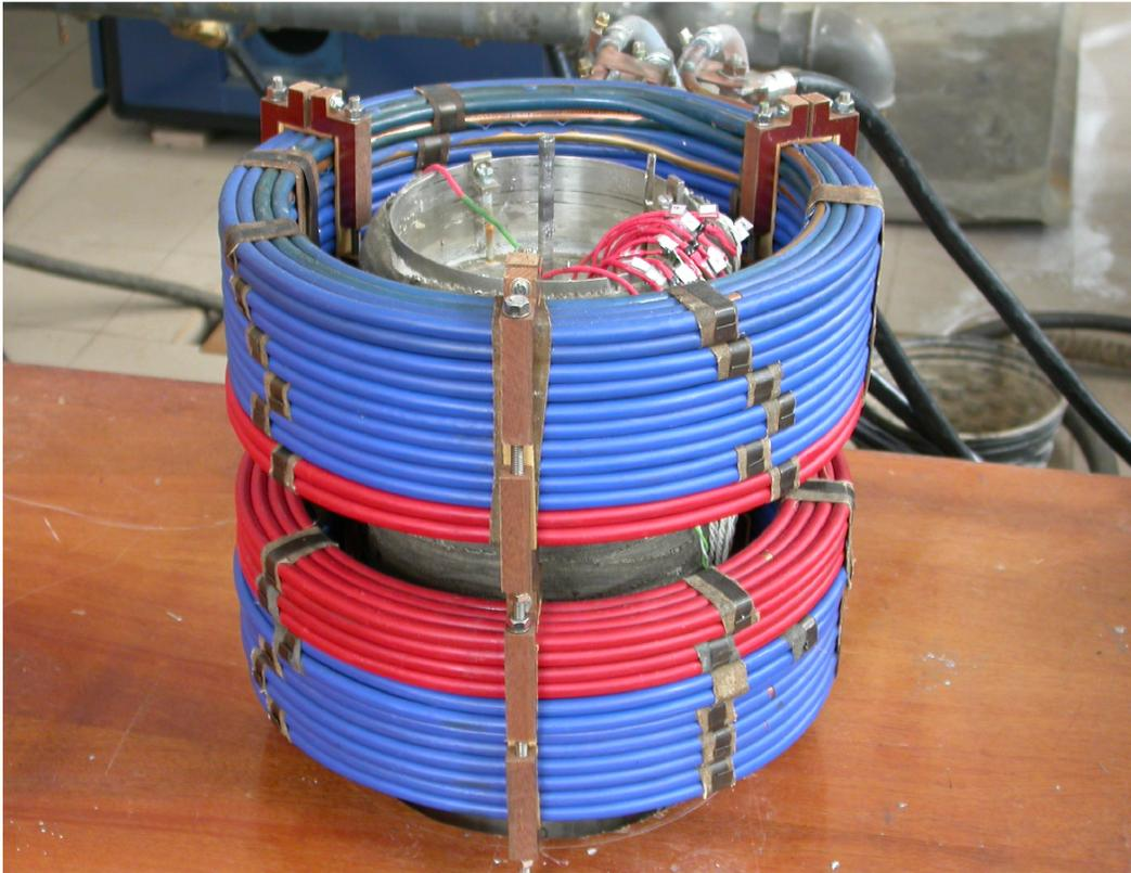
**Fig. 4** Inductor of magnetic fields.
