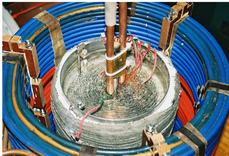
**Fig. 3** Gallium cell with water-cooling system.
